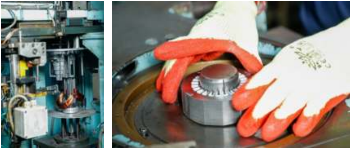
Automatic Winding. We are equipped with a coil insertion machine which enables automatic slot insulation, formation of coil sets and insertion of coil sets in the stator.
