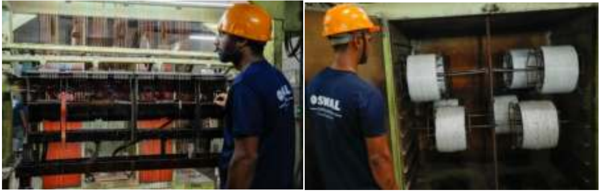
Cable Manufacturing. We manufacture PVC flat cables by extruding multi-strand copper conductors insulated with a PVC compound that is resistant to grease, oil, and water.
