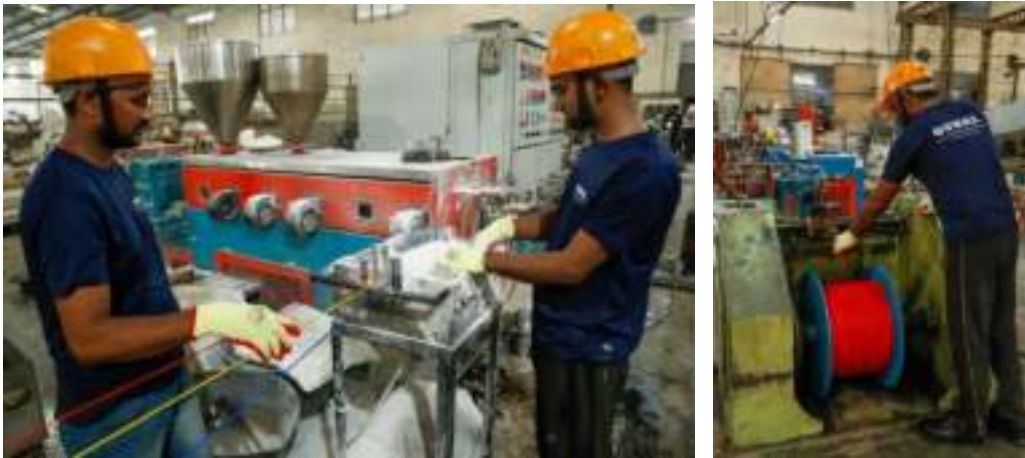
Cable Manufacturing. We manufacture PVC flat cables by extruding multi-strand copper conductors insulated with a PVC compound that is resistant to grease, oil, and water.
