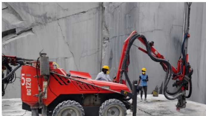
Drill machine equipped with dust sucking mechanism
